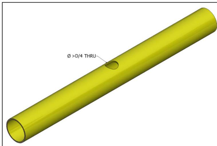
**Figure 5: Simple puncture (structural)**
