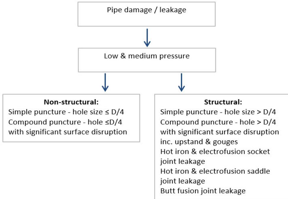
**Figure 1 Damage type classification**
