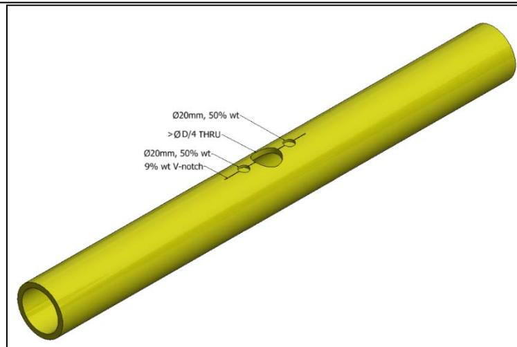
**Figure 6: Compound puncture (structural)**
