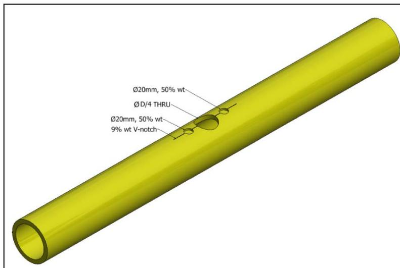
**Figure 4: Compound puncture (non-structural)**
