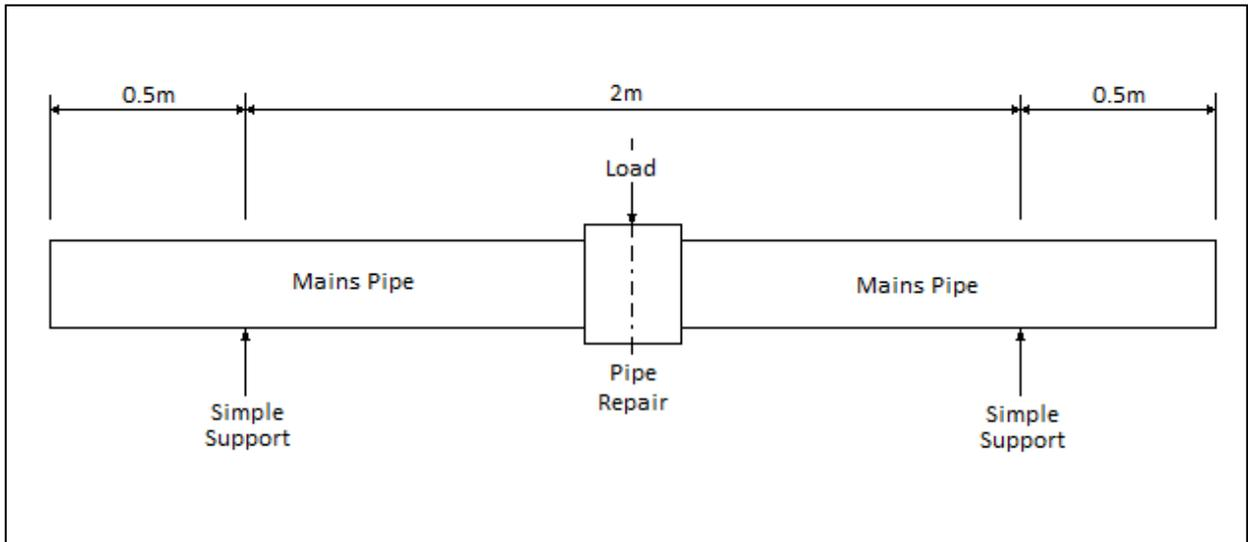
**Figure 14 Pipe bending**
