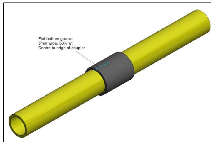
**Figure 7: Hot-iron & EF socket joint leakage (structural)**
