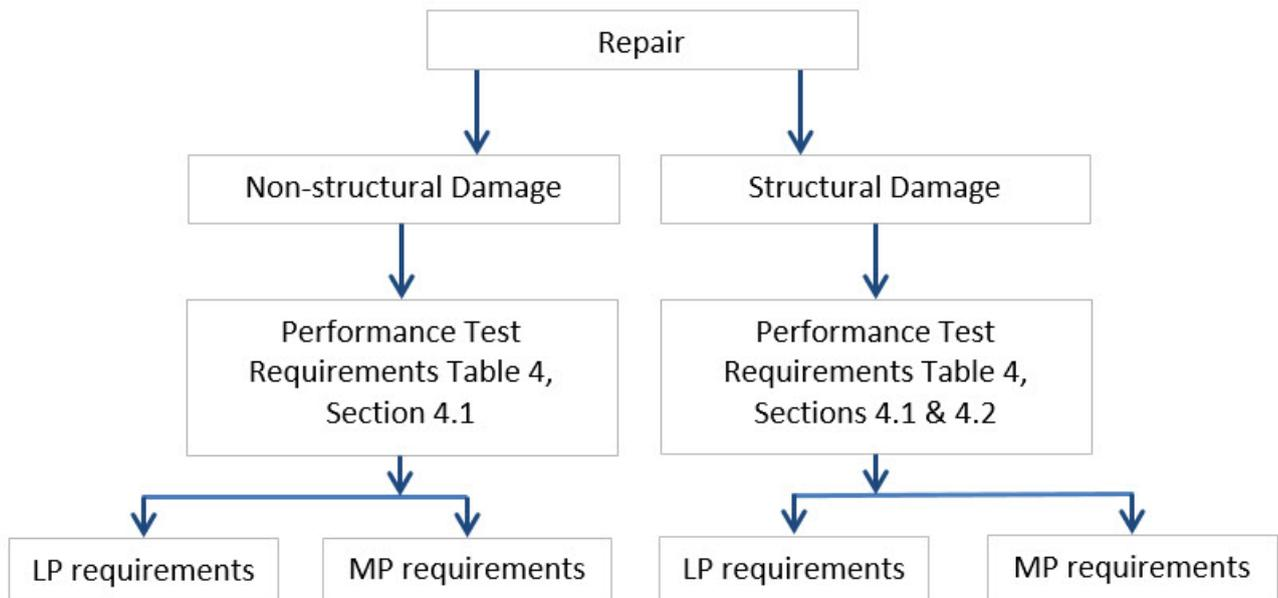
**Figure 2 PE repair test requirements**
