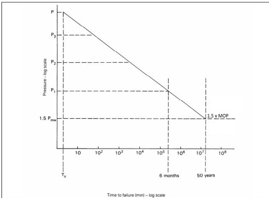
**Figure 10 Pressure life testing (GIS/LC1)**
