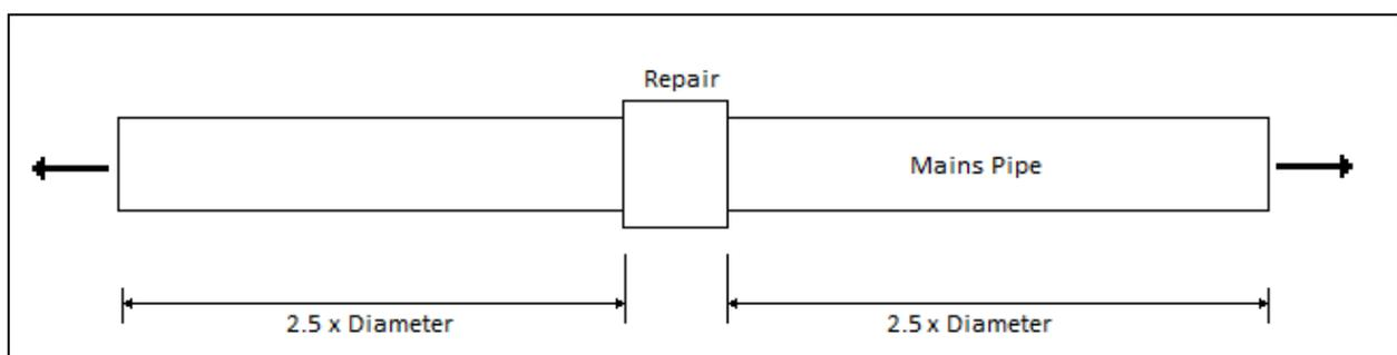
**Figure 16** End load resistance
