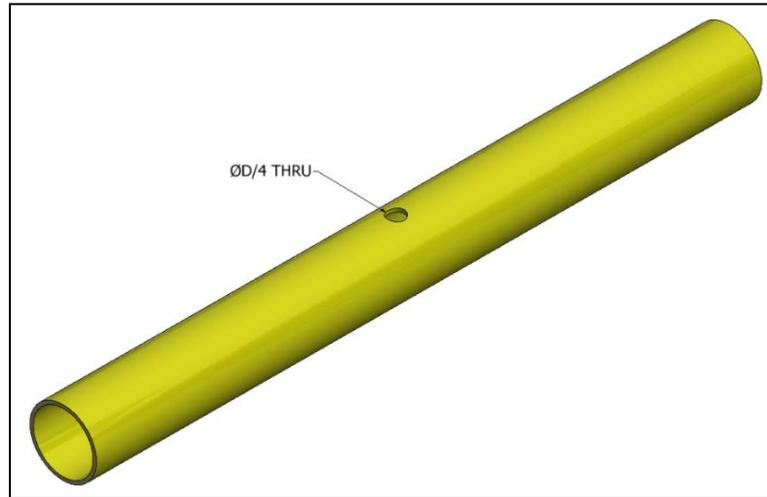
**Figure 3: Simple puncture (non-structural)**
