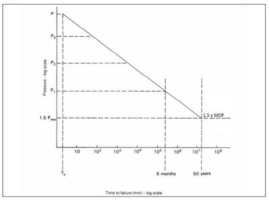
Figure 10 Pressure life testing (GIS/LC1)
