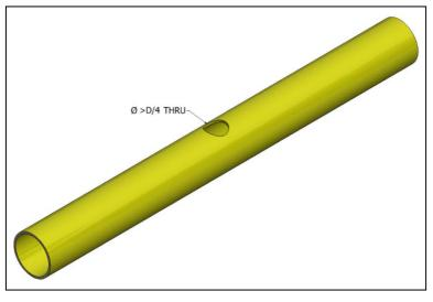
Figure 5: Simple puncture (structural)
