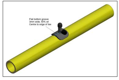
Figure 8: Hot-iron & EF saddle joint leakage (structural)
