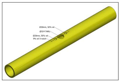
Figure 4: Compound puncture (non-structural)
