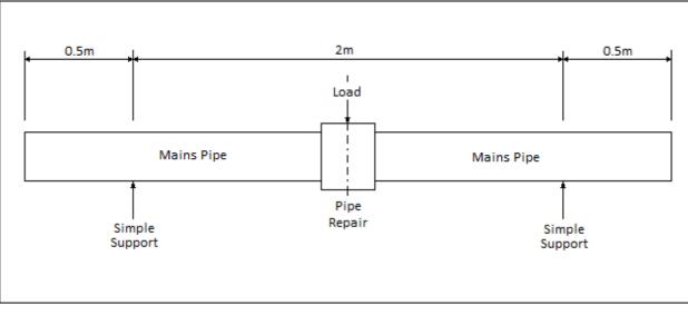
Figure 13 Pipe vibration
