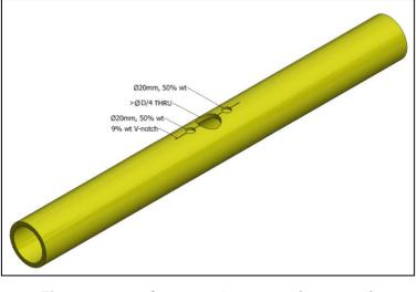
Figure 6: Compound puncture (structural)
