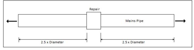
Figure 16 End load resistance
