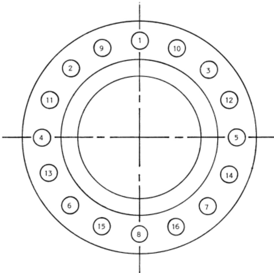
**Figure 2: Typical Bolt Tightening Sequence (2)**
