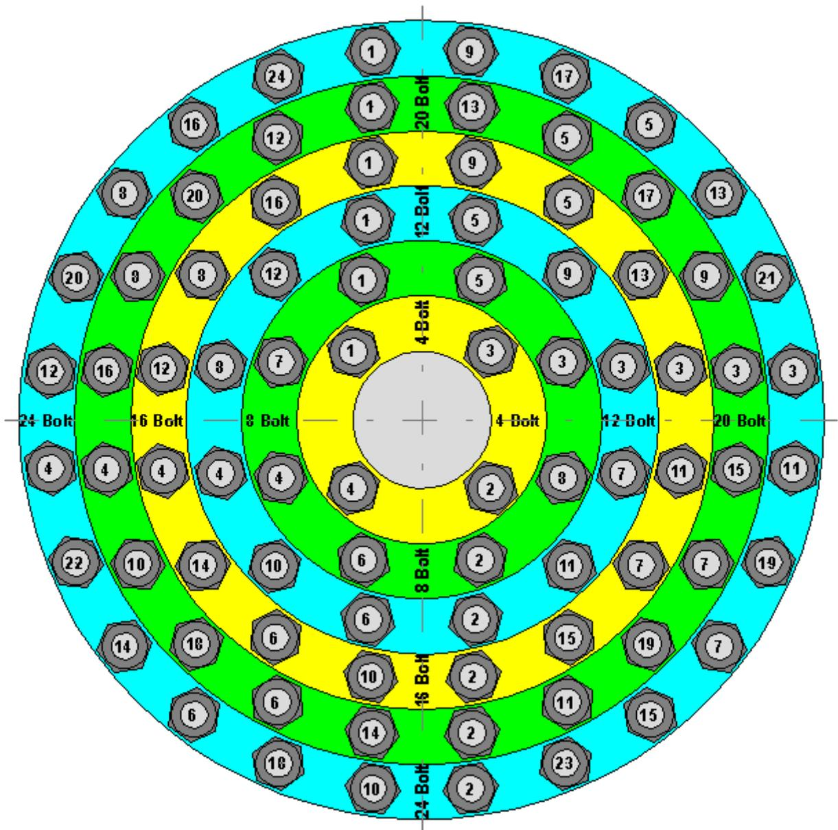
Figure 1: Typical Bolt Tightening Sequence (1)
