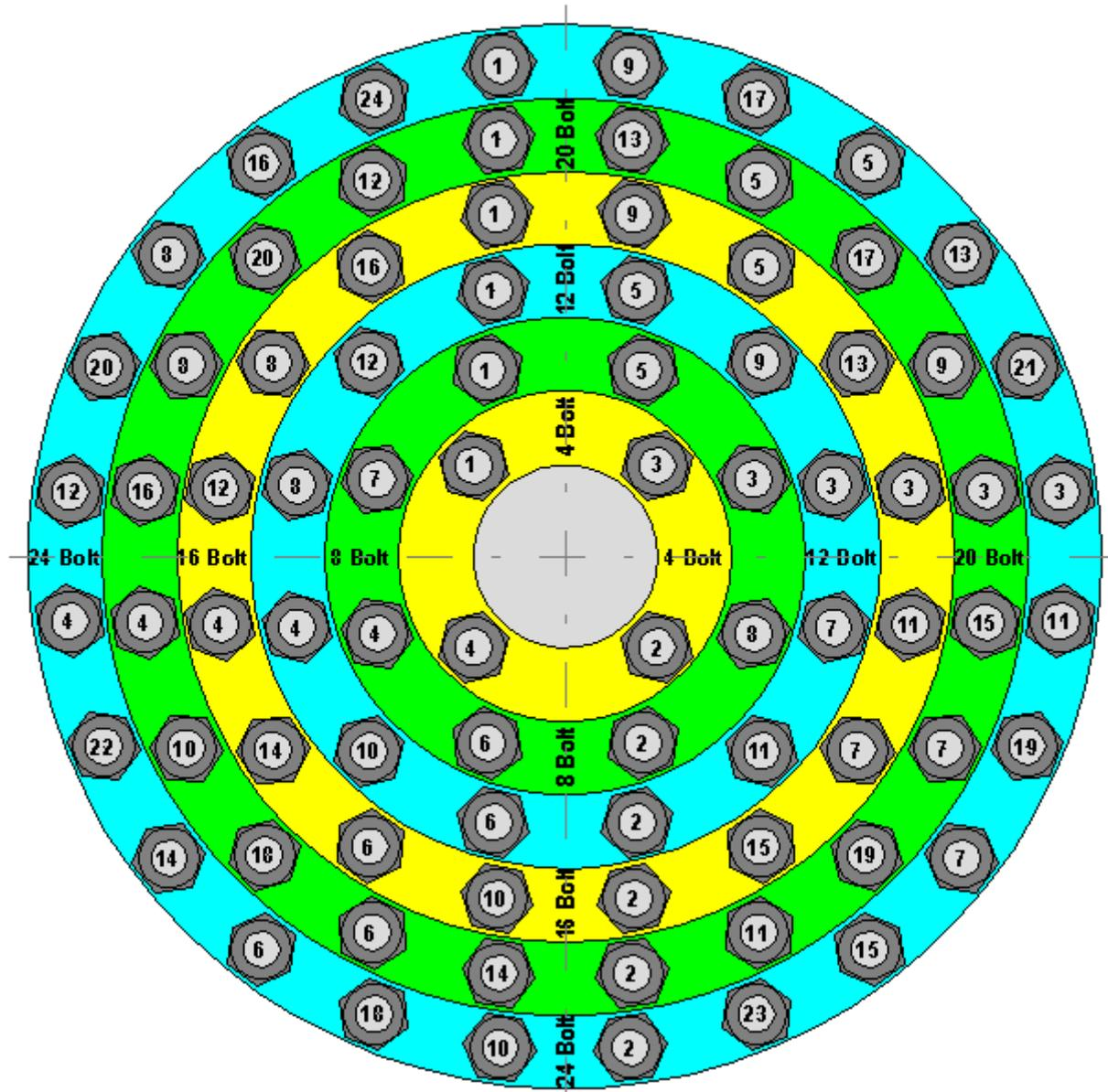
Figure 3: Typical Bolt Tightening Sequence
