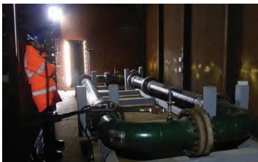
FIGURE 3 FLOW LOOP TRIAL IN HYDROGEN-RICH GAS MIX AT DNV GL SPADEADAM
