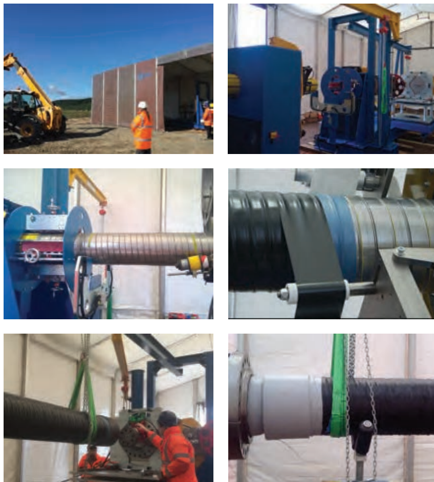
FIGURE 2 MOBILE PIPE FABRICATION AT THE FIELD TRIAL SITE
